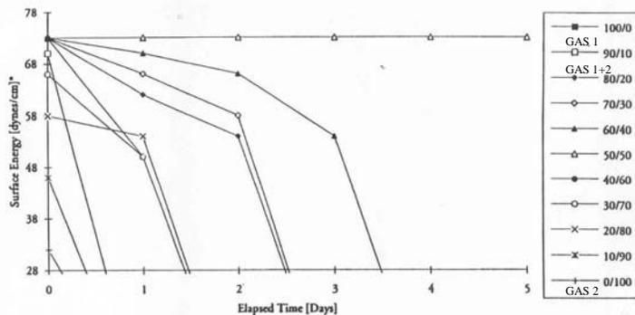
Figure 3. Change in surface energy based on gas mixture
