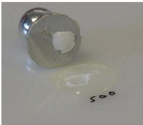
**Figure 3: HDPE Pull Out**
