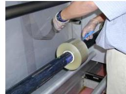
Figure 5. Operator shown removing treated film from roll-to-roll system
