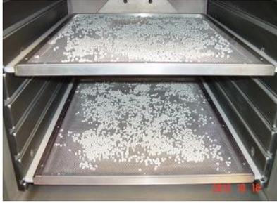
Figure 1. Porous polyethylene caps loaded on trays for chemistry discovery trials.
