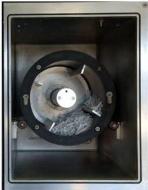
Figure 2. PS0500 Tumbler System loaded with polyethylene filters
