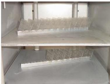
Figure 3. PS0500 system loaded with microfluidic cartridges
