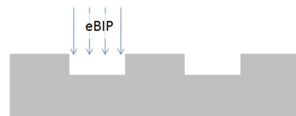
Fig. 1b: Selective plasma exposure using electron-beam induced plasmas (eBIP) – no masking required
