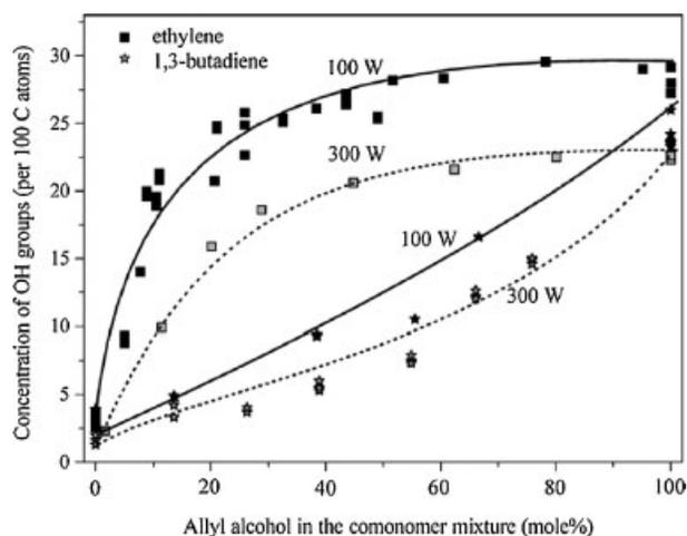
Figure 5. Densities of OH groups on ethylene/allyl alcohol and butadiene/allyl alcohol copolymers measured by XPS and derivatization with TFSA. Reproduced with permission from ref.<sup>[144]</sup>
