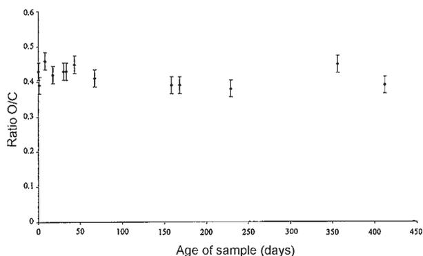
Figure 8. O/C ratio of acrylic acid plasma polymer as a function of sample age. Reprinted with permission from ref.<sup>[116]</sup>
