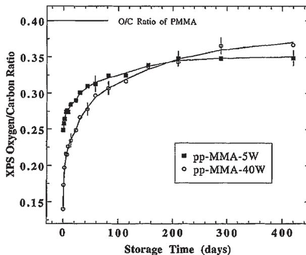
Figure 9. XPS O/C ratios (0° emission) as a function of storage time, of plasma-polymerized methyl methacrylate deposited at power levels of 5 and 40 W. Also included is the theoretical value of O/C for PMMA (0.4). Error bars represent one standard deviation. Reproduced with permission from ref.<sup>[118]</sup>
