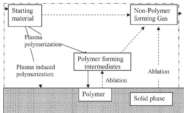
Figure 1. Schematic diagram of competitive ablation polymerization, reproduced from ref. <sup>[1]</sup> and <sup>[2]</sup>.
